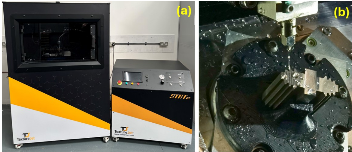
Figure 1. (a) TextureJet's Stat ® system (right) coupled with PrecisionJet 5-axis automation system (left), which has been developed to create controllable and repeatable edge breaks on any conductive material. (b) Stat ® System being utilised to edge break complex geometry.
